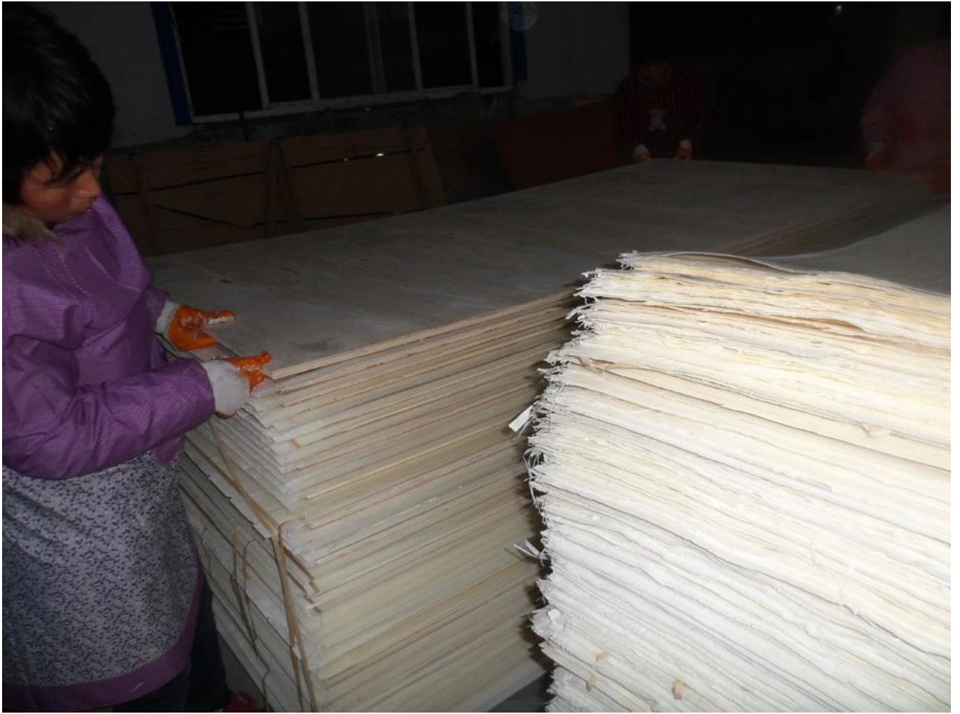
Putting the base plywood on the veneer and MDF
