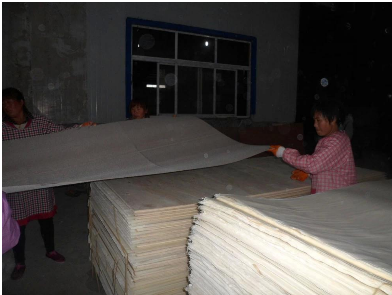
The MDF boards have been painted well by the glue,the veneers have been put on the back.
