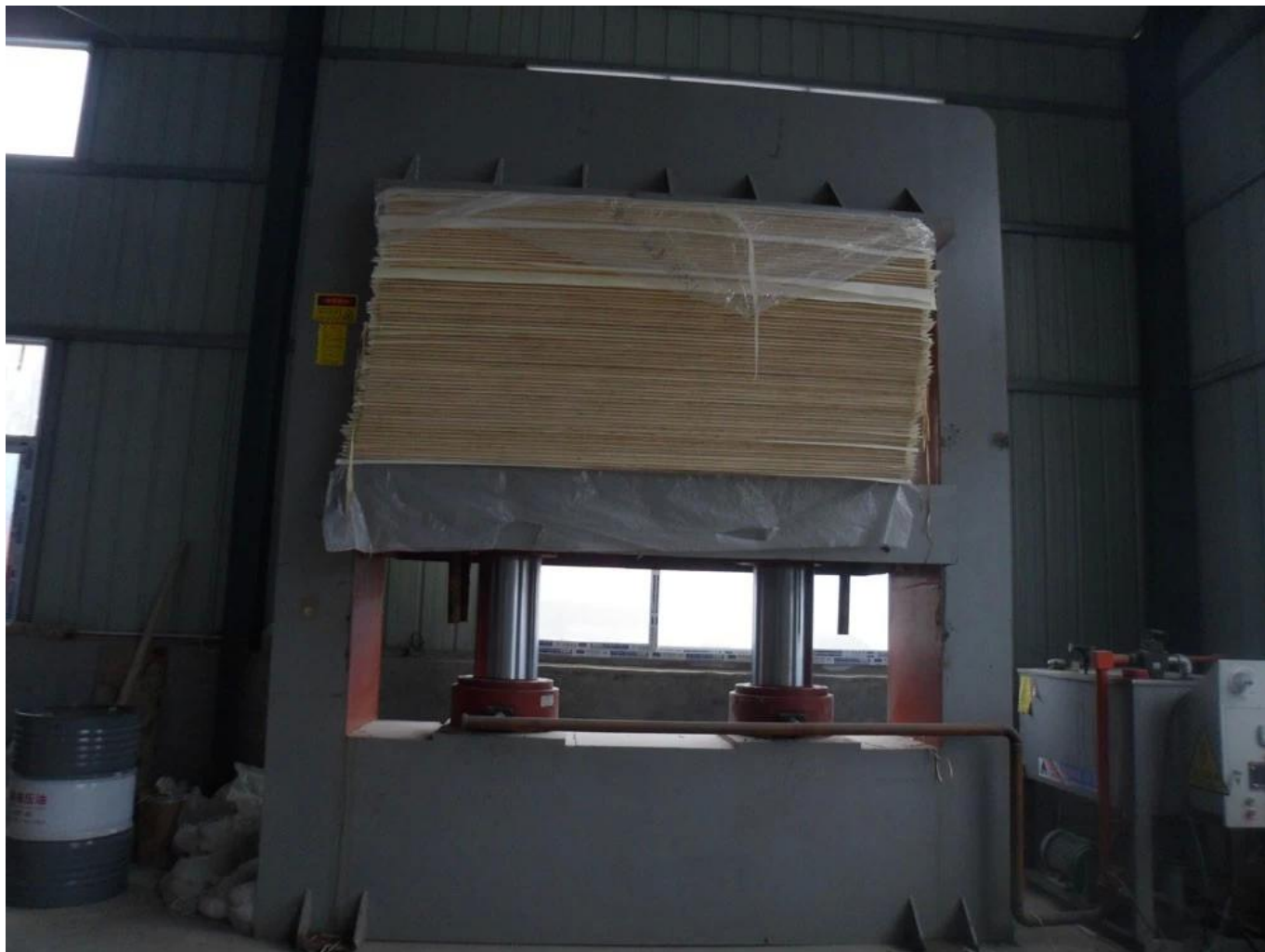
After covered the MDF and poplar veneer,will be cold-pressing firstly
