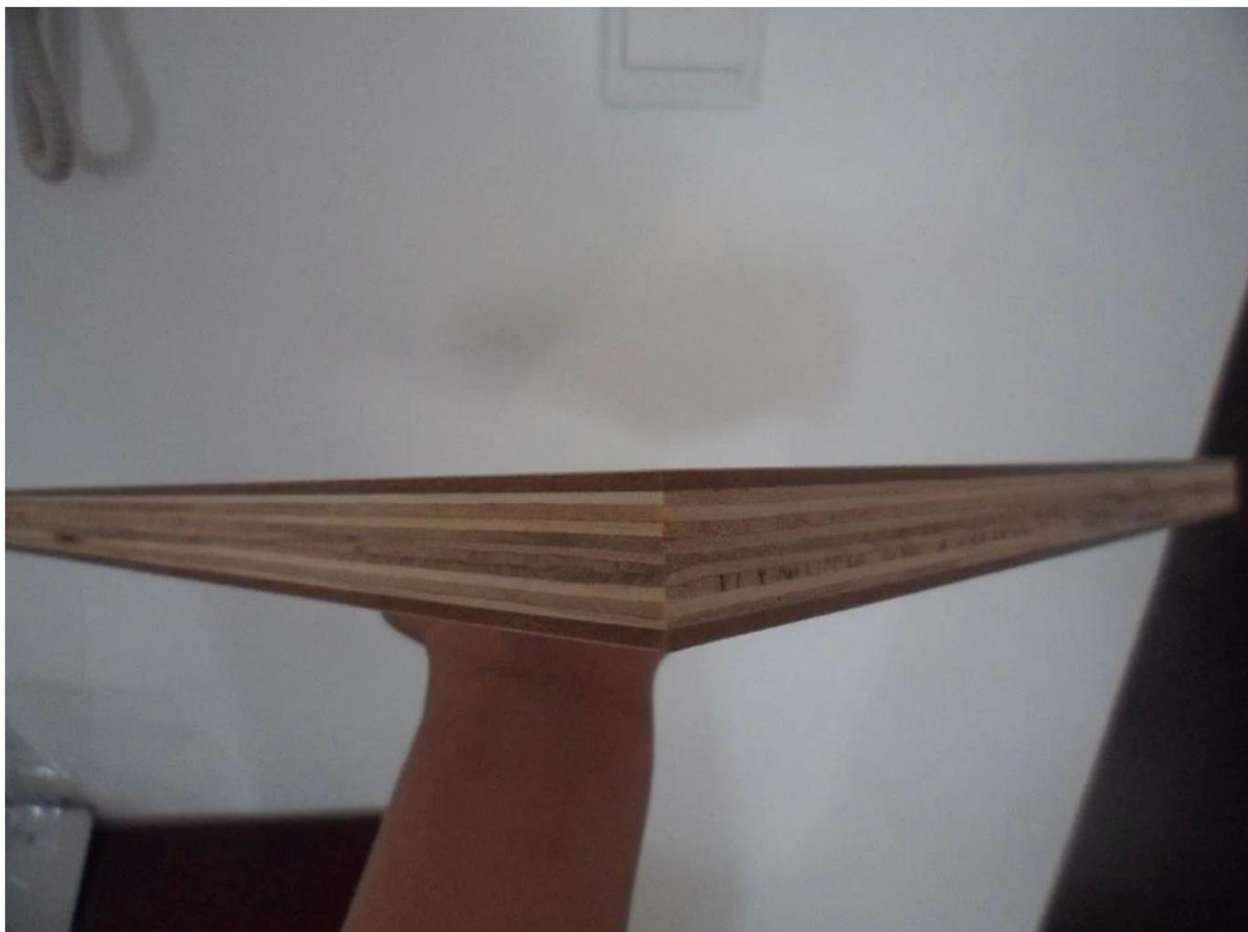
you can see clearly from the images that there are two layers of MDF on both sides, these two MDF could perfectly protect from breaking lines lines of paint lines of knife, keep the color consistent when you make the furniture, they could solve everything
